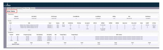
Note: The S11 server is with automatic frequency adjustment. Firmware will stop running when the Temp(PCB) reaches to 95°C, there will be an error message "Fatal Error: Temperature is too high!" shown in the bottom of kernel log page.
